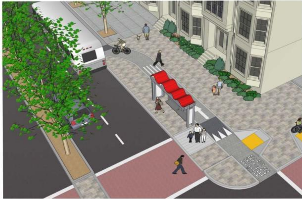
Proposed "Bus Bulb Plaza" seeks to reduce conflict between bikes and buses at bus stops
