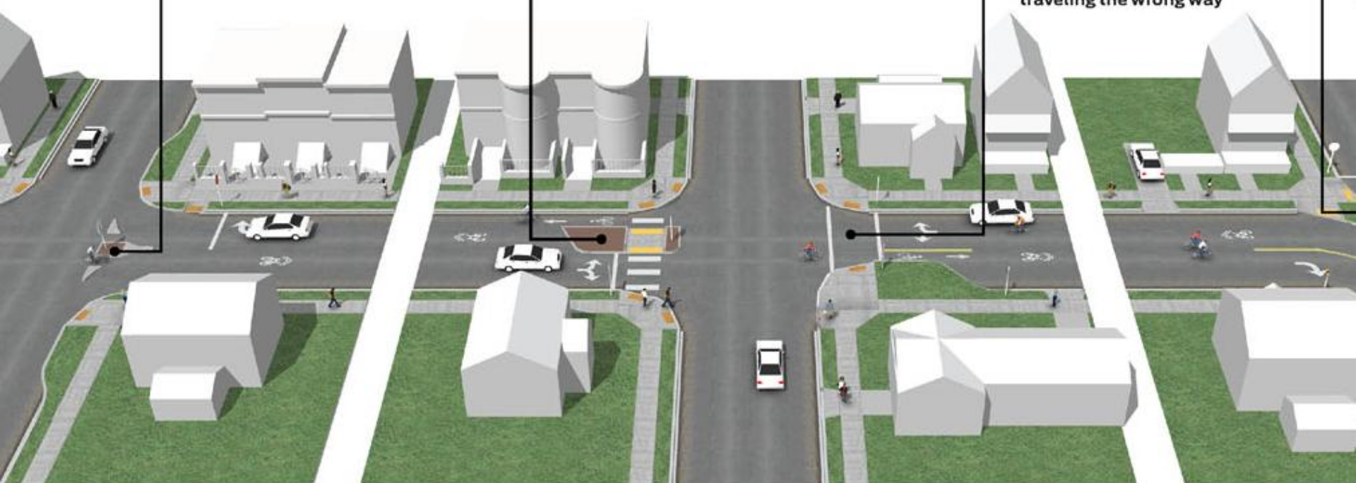
Partial Closure (Edge Island with Pass Through)
