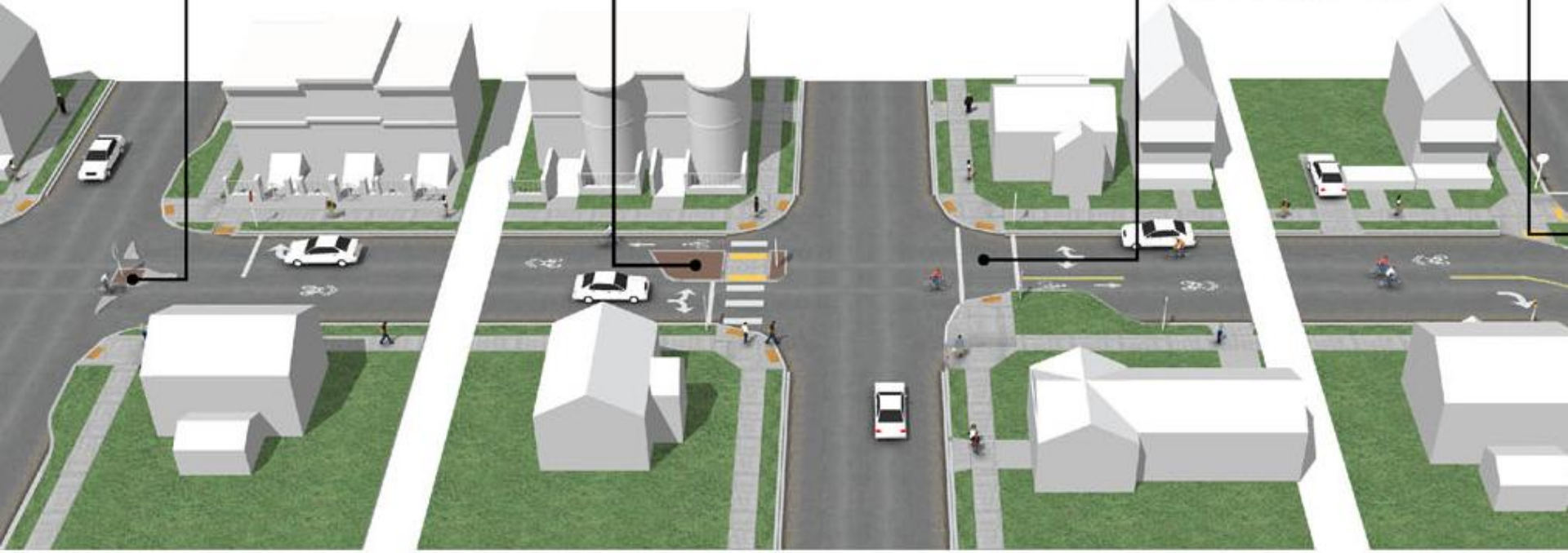
Partial Closure (Edge Island with Pass Through)
